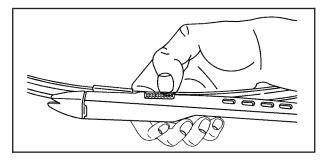
Squeeze the tabs on each side of the wiper blade assembly and slide the assembly off the end of the wiper arm.
